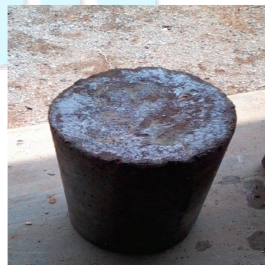
Figure 4.3: Specimen under attack by Sulphate
