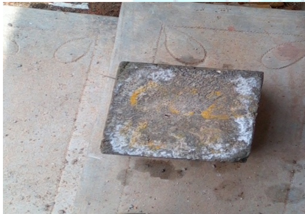
Figure 4.1 Specimen under attack of Sulphate
